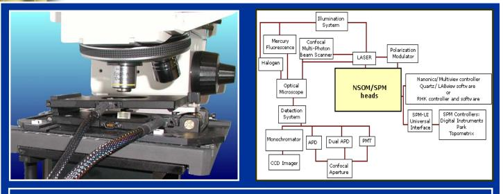
• The central part of NSOM is the tapered, aluminum coated, single-mode optical fiber probe (tip), which has a tiny aperture of only a few tens of nanometers. High optical resolution is achieved by illuminating a sample through the sub-wavelength aperture while the sample is held in close proximity to the probe. Within the near-field the optical resolution is limited only by the probe aperture size (~ 50 nm), breaking the diffraction limit (I/2) to the resolution of ordinary optical microscopy
